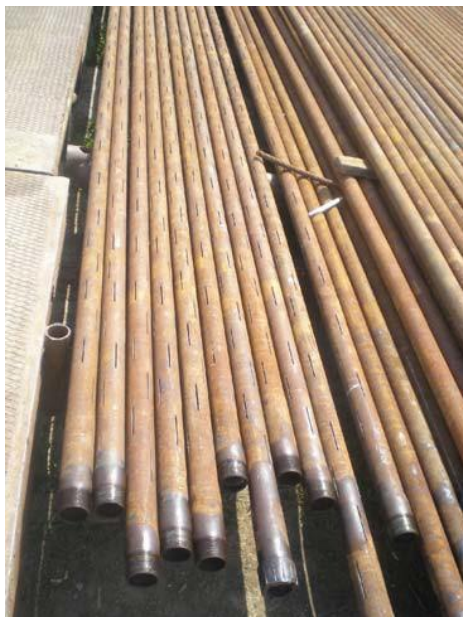
Figure 12: Filter – perforated casing tubes
