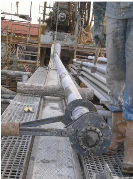
Figure 5: Core drilled using the GEOBOR S double core barrel
