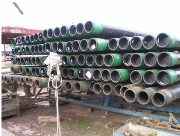
Figure 2: 7" Tubes used for casing the PVGT – LT1borehole
