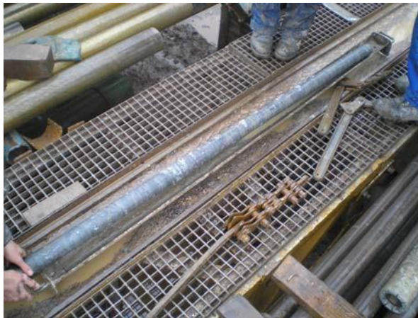
Figure 5: Core drilled using the GEOBOR S double core barrel
