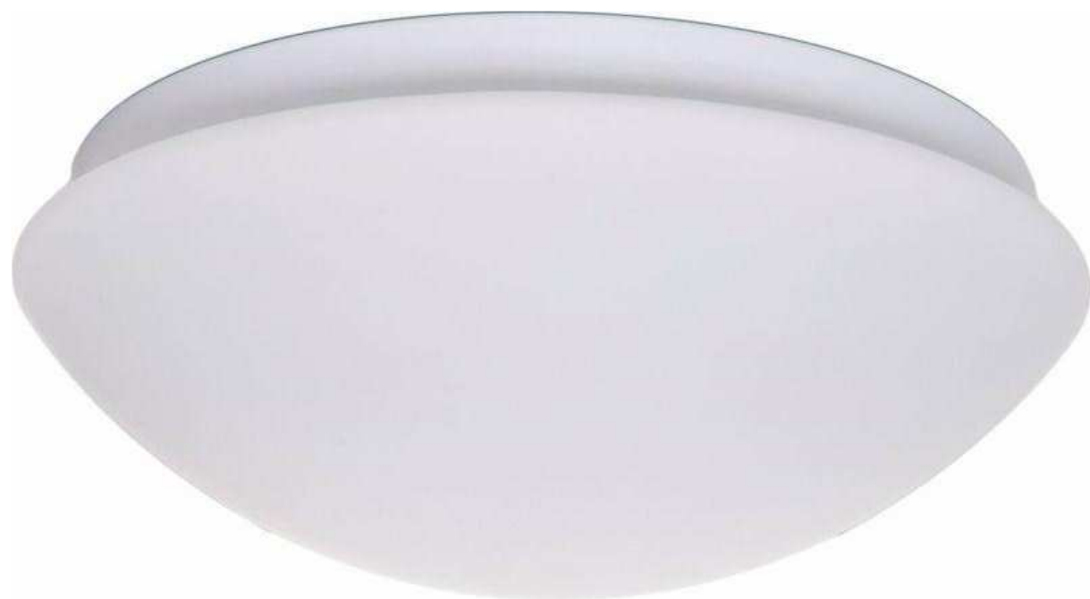
SVÍTIDLO "B" - SVÍTIDLO LED PR.380mm, 16W, 1380lm, 2700K, IP44
